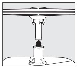
■ Lift up on the <u>lower</u> spray arm to remove it.
